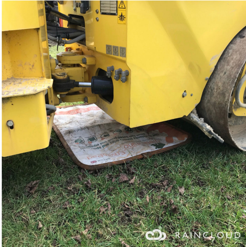
Plate 12 and Plate 13: Drip trays and pads to limit uncontained chemical spillages
